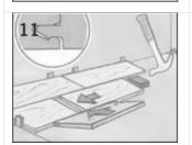
Use a 4"-6" piece to hold the tongue and groove on the same plane, limit end joint damage and ensure planks engage square. Tap end joints with multiple light taps, striking the tapping block eveny until end joints close. NOTE: Tapping too hard or striking the tapping block unevenly can result in installation-related damage or peaking.
