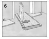
Remove the tongue on the panels that face the walls to allow room for spacers and prevent problems from spills.
