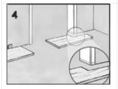
If possible, start to lay panels under the door jam and finish installing planks on a wall without a door jam. See "Working with Limited Clearance" section.
