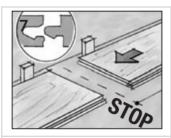
Lay panels close together on the floor.
